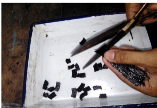
2.2 Cutting the fibre(by own camera)
