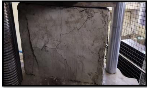
Fig: Wall after testing
