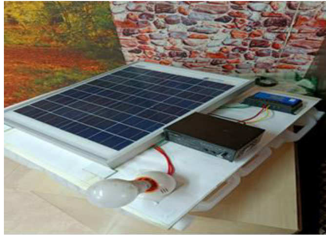
Figure 5 a prototype of floating solar plant of 20 w capacity with recycled plastic cans
