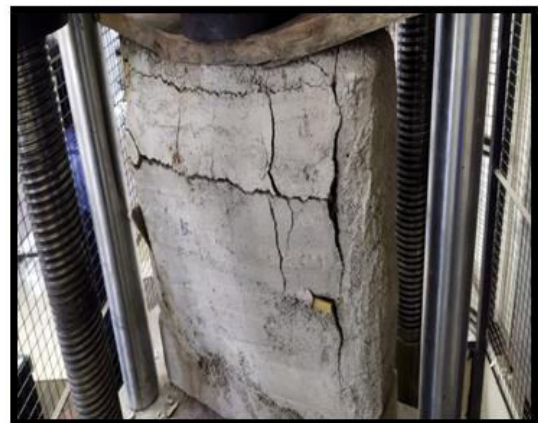
Fig : After Testing
