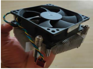
Fig.1 Heatsink attached with Fan.
