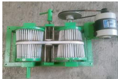
Figure 1 Test rig of Positive engagement Variable speed drive
